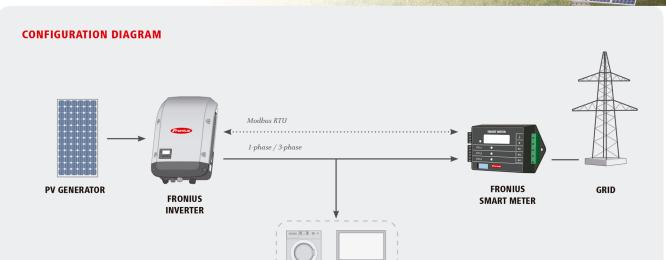
The Fronius Smart Meter is compatible with all inverters with an RS485 interface (Modbus RTU). The Fronius Smart Meter works in conjunction with the Fronius Datamanager 2.0 for the Fronius IG Plus inverters. The Fronius Smart Meter can be retrofitted at any time together with the Fronius Datamanager 2.0 in inverters that have already been installed.
